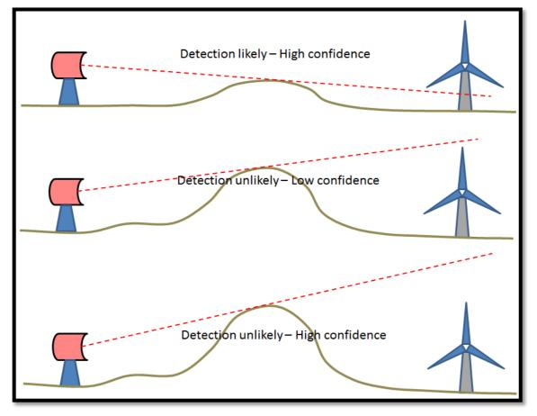
Diffraction is a physical effect that means radio signals passing just above the blocking point are weakened and that weak radio signals radiate below the blocking point. Standard line of sight
