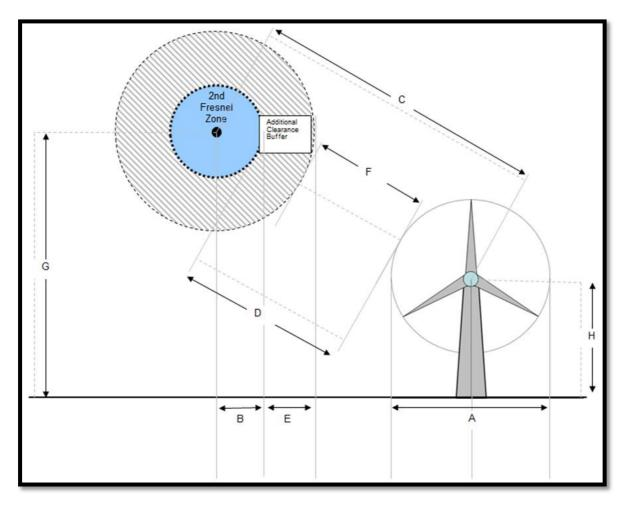
Terrain based assessments can also be used to determine whether a radio communications link between two sites will work reliably by determining whether the link path and the zone around it are clear of terrain and obstructions. The required clearance is dependent on the frequency of the radio link. It is also possible to predict radio coverage from a specific transmitter over a particular area. More complex assessments can predict interference from wind turbines over a specific area.
